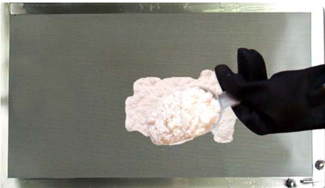
Applying filter powder to screen.
